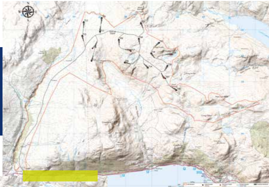
Post Scoping Design – 18 wind turbine locations, indicative access tracks and hardstandings added.
