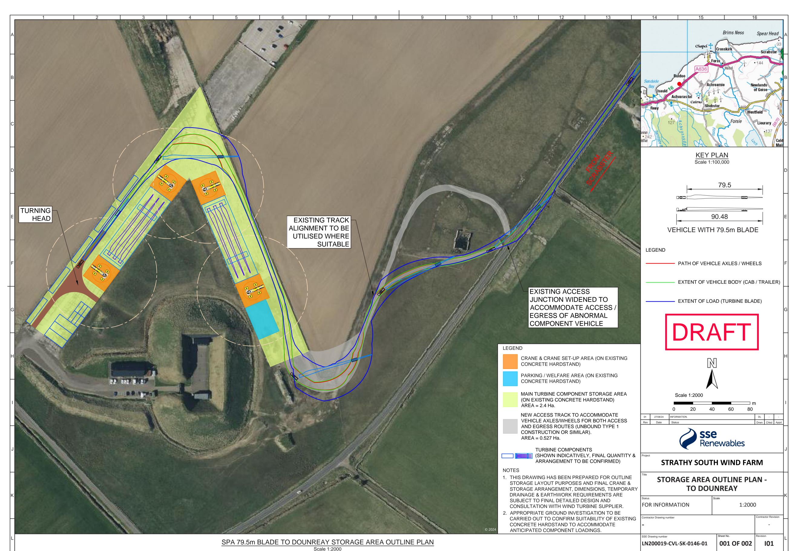
Drawing prepared for outline storage purposes only. Final crane and storage arrangement, dimensions, temporary drainage and earthwork requirements are subject to final detailed design and consultation with the wind turbine supplier.
